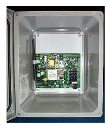
Typical examples show RFScada devices with license free ISM modules and internal antennas installed. On the left is the lower powered version, and the higher powered (SS1) version is on the right.
