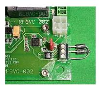
As a final precaution when using extreme cable lengths a 100 Ohm resistor is sometimes installed in series with the shield between
