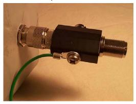
arrestor may be mounted inside the cabinet required; ensure that the surge arrestor case or block is securely grounded directly to the main input ground or ground rod. The surge arrestor has field replaceable element, to access it remove the screw on the side of the
